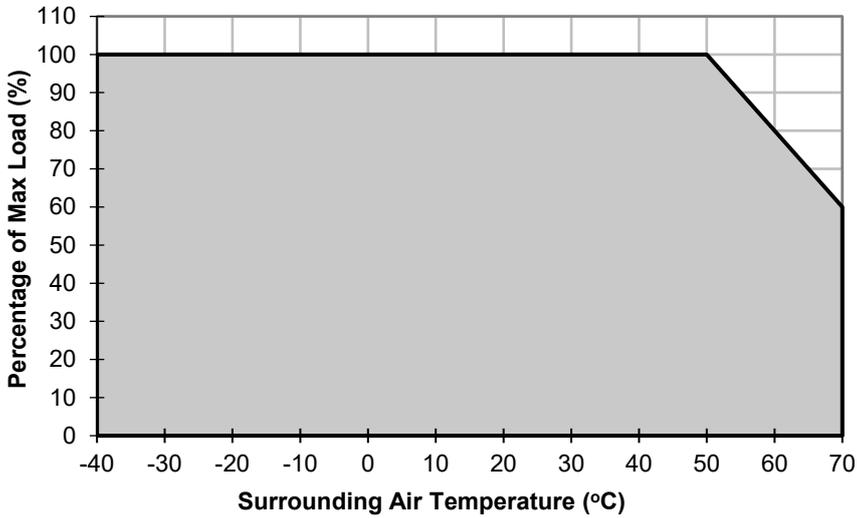
**Fig. 1 De-rating for Horizontal Mounting Orientation**
