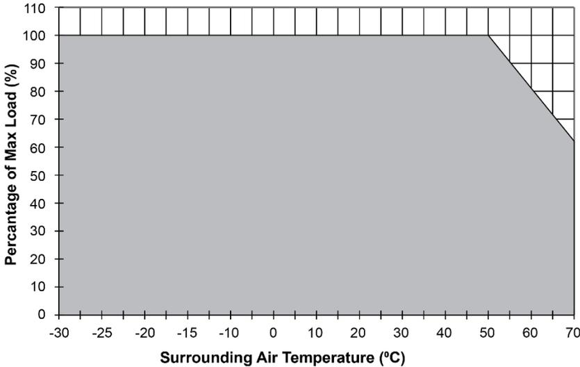
**Fig. 1 De-rating for Horizontal Mounting Orientation**
