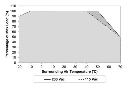
Fig. 1 De-rating for Vertical Mounting Orientation
