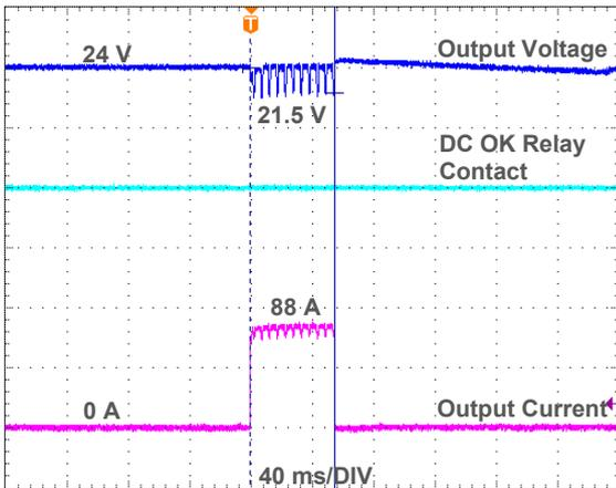
Fig. 8.1 APB 200% of nominal output current for 50 ms
