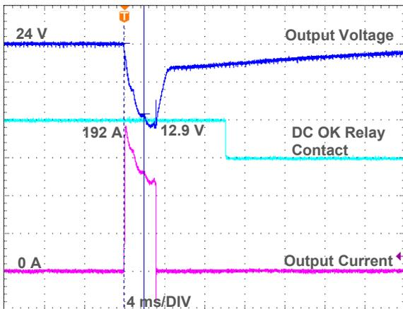
Fig. 8.3 APB 500% of nominal output current for 2 ms
