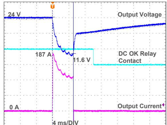
Fig. 8.4 APB 500% of nominal output current for 5 ms
