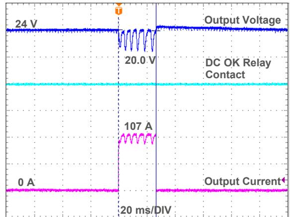
Fig. 8.2 APB 275% of nominal output current for 25 ms
