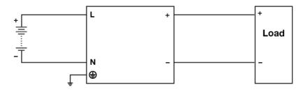
Fig. 4 DC Input Operation Connection Diagram
