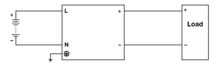
Fig. 4 DC Input Operation Connection Diagram
