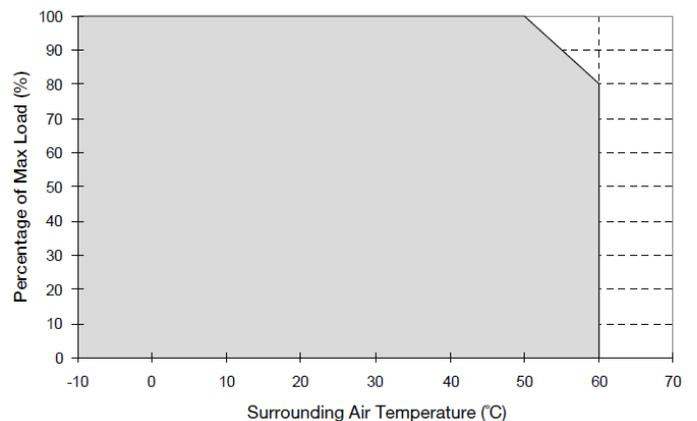
Fig.1.4 De-rating for Mounting Orientation A to F
