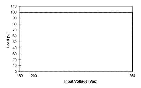
Fig. 2 De-rating for AC Input Voltage
