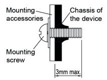
Fig. 4 Mounting Screw
