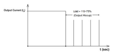
It is not recommended to prolong the duration of lo when it is <110% but >100%, since it may cause damage to the PSU.
