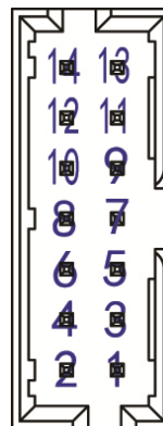
Fig. 6: Signal port and Auxiliary DC Output (CN602) – Pin assignment
