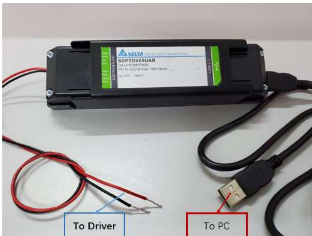
Figure 2. The picture of the DMX512&RDM programming tool
