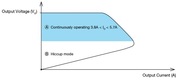
Additionally, if the  $I_o$  is  $>102\sim 108\%$  for a prolonged period of time (depending on the load), the Over Temperature Protection (OTP) will be activated due to high temperature on critical components. The power supply will then go into "Latch mode" until the PSU cools down and the AC power is recycled.
