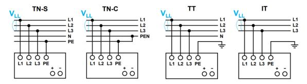
Fig. 4 AC Input Operation Connection Diagram
