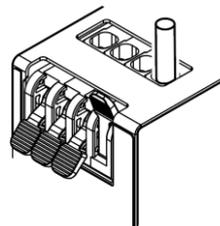
To disconnect the wires, reverse the procedure. Flexible cables require ferrules.
