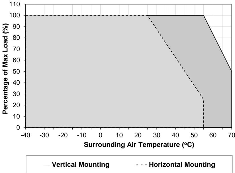
**Fig. 1 De-rating for Vertical Mounting Orientation**
