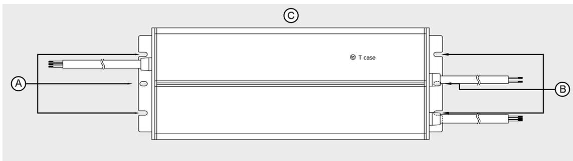
Fig. 3 Mounting Hole Locations
