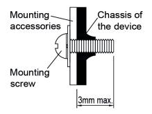
■ For PMT Series (Refer to Fig. 4): Only use M3 screw ≤ 3 mm (0.20 inch) through the base mounting holes. This is to keep a safe distance between the screw and internal components. Recommended mounting tightening torque: 4~7 Kgf.cm.
