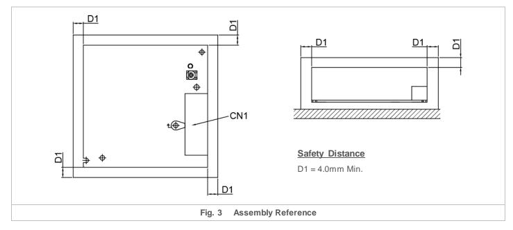
Ensure the mounted device is kept at  $\geq$  4 mm (0.16 inch) safety distance at all sides from other components and equipments. In addition, to ensure sufficient convection cooling, always maintain a distance of  $\geq$  20 mm (0.79 inch) from ventilated surfaces while the device is in operation.
